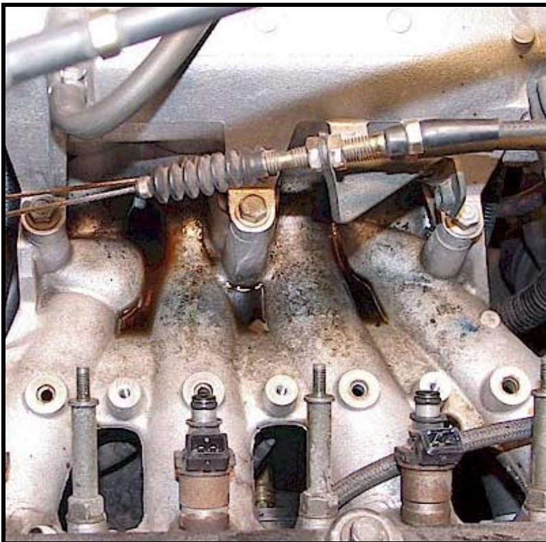
Here is a picture of all 4 ports cleaned up and ready for re-assembly. Cleaning is best done with a pick and then a bottle type wire brush.
