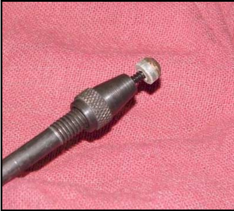
A picture of an EGR passage port still attached to the slide hammer.
